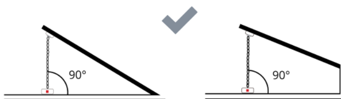
Chain perpendicular/90° to the magnet face
